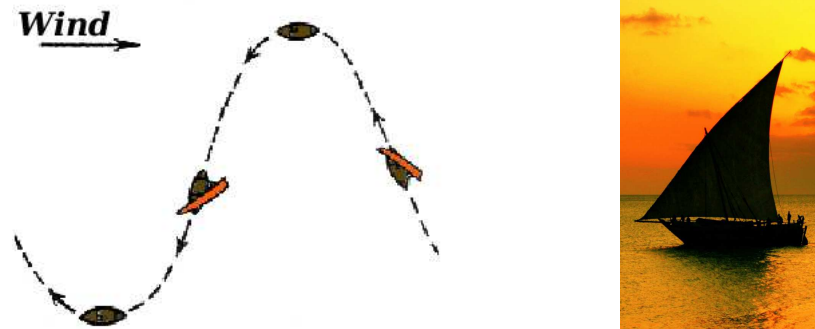
Figure 5.1: A triangular sail atop a traditional Arab sailing vessel, the dhow (right). Older square sails permitted sailing only before the wind. But the efficient lateen sail worked like a wing (with high pressure on one side and low pressure on the other), allowing a ship to go almost directly into a headwind. By tacking , in a zig-zag pattern, it became possible to sail in any direction, provided there was some wind at all (left). For centuries seafarers expertly combined both sails to traverse extensive distances, greatly increasing the reach of medieval navigation. (Partially adapted from http://www.britannica.com/EBchecked/topic/331395 , http://allitera.tive.org/archives/004922.html and http://landscapedvd.com/desktops/images/ship1280x1024.jpg .)
